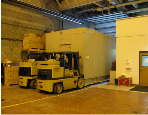
Above left, moving a General Electric EX-2100 exciter house with LCI for inspection.
